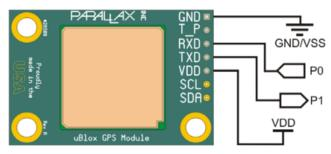
The PAM-7Q GPS Module can be interfaced with many common microcontrollers or computers, including the Propeller, BASIC Stamp, Arduino, PIC, Raspberry Pi, Beaglebone, and more. At minimum, you can
